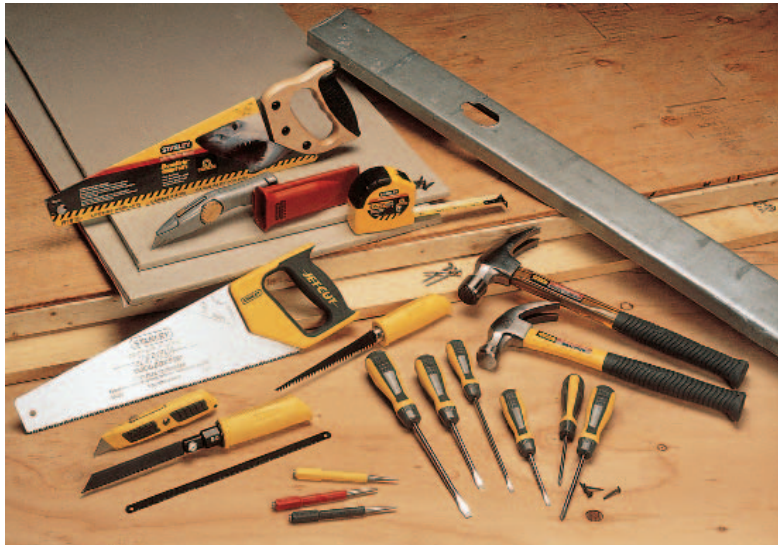
Figure 3-9 Ergonomic Tools Design for Safety The ergonomic design of tools increases their usability. Some tools shown here have cushioned handles while others are shaped in a way that reduces wrist strain. Why do you think the shape of a tool can make a hand tool safer or easier to use?
