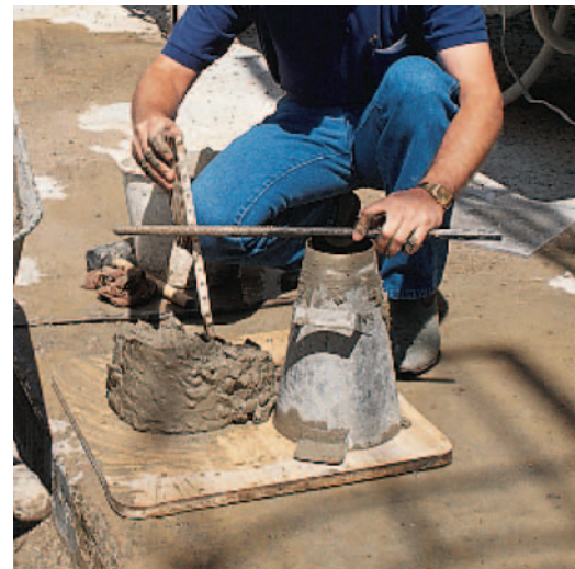
Figure 8-6 Testing Slump Reading Slump When the cone is removed from the concrete, the resulting slump is determined by measuring from a rod to the top of the concrete.
