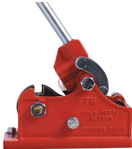
Figure 8-9 A Rebar Shear Cutting Leverage The long handle of this rebar shear provides enough leverage for smooth cuts.
