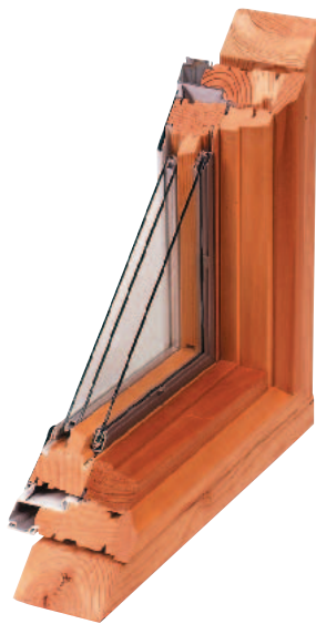
Figure 20-12 Insulating Glass Window Double Glazed A cross section of an insulating glass window.
