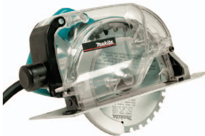
Figure 23-31 Fiber Cement Dust Collection Safety Feature The clear housing on this circular saw helps to contain the fine dust created when fiber cement products are cut.
