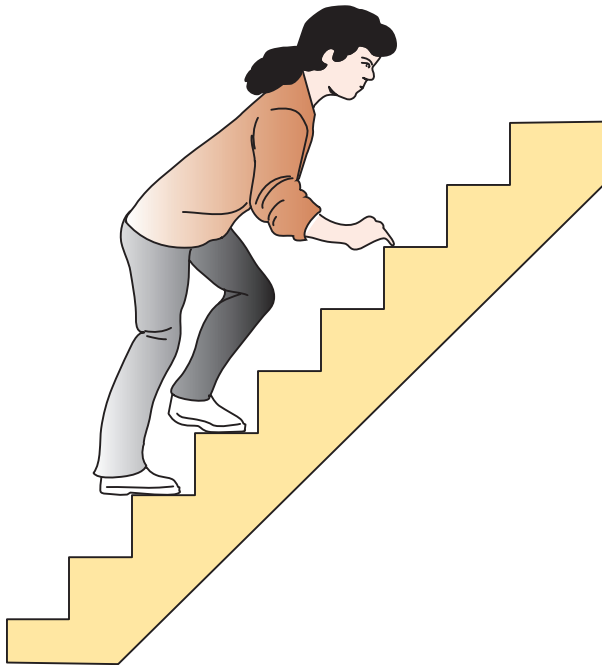
Figure 25-9 Stair Comfort Too Steep A stairway should be built with the proper height of risers and treads. On this stairway, the tread is too shallow and the riser is too high.
