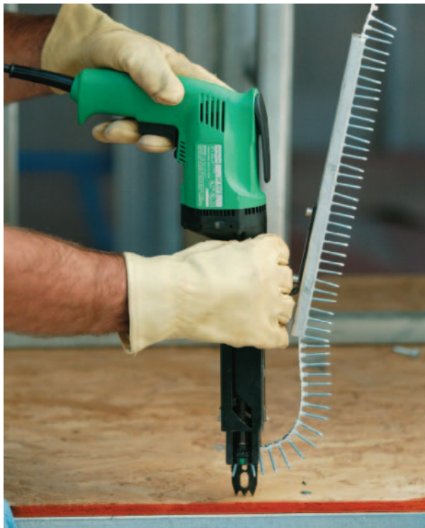
Figure 29-4 Collated Screws Feathering Strips Using an attachment that feeds collated screws into the screw gun.
