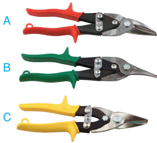
Figure 29-14 Aviation Snips Right or Left A. Red-handled aviation snips are for right-handed people. B. Green-handled snips are for left-handed people. C. Yellow-handled snips should be used for straight cuts.
