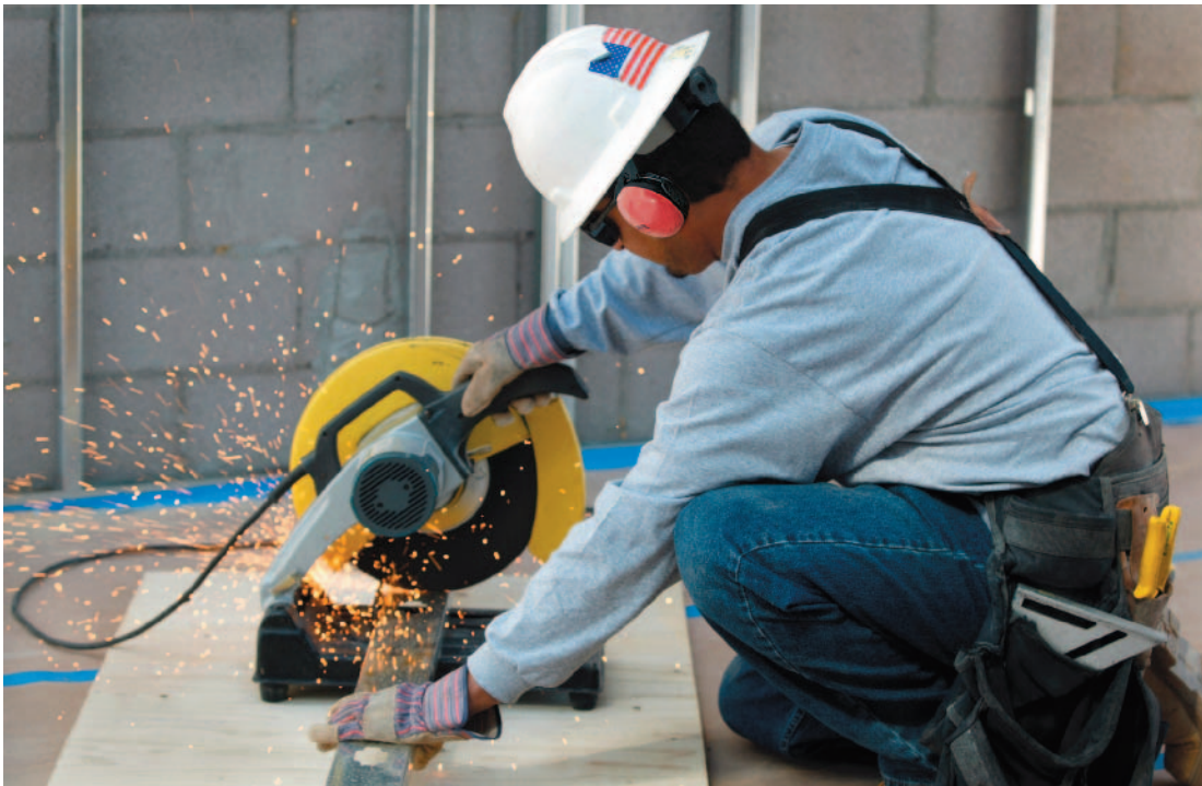
Figure 29-9 Chop Saw Abrasive Blade These tools are used for cutting metal.
