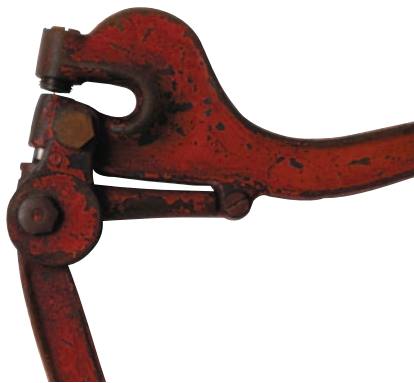
Figure 29-15 Hole Punch Packs a Punch A hole punch makes holes in steel members.
