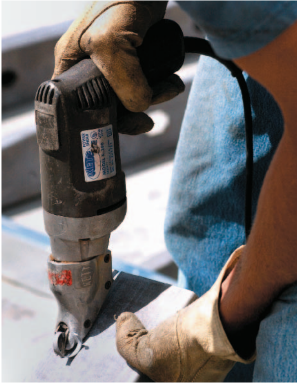
Figure 29-8 Electric Shears Cutting Steel Electric shears can cut sheet steel.
