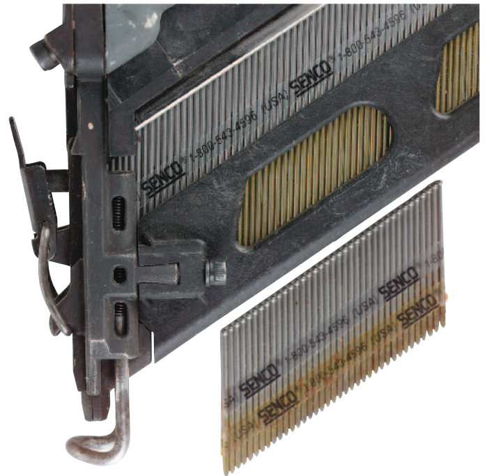
Figure 29-21 Collated Drive Pins Drive Pins Collated drive pins used with a pneumatic nailer.
