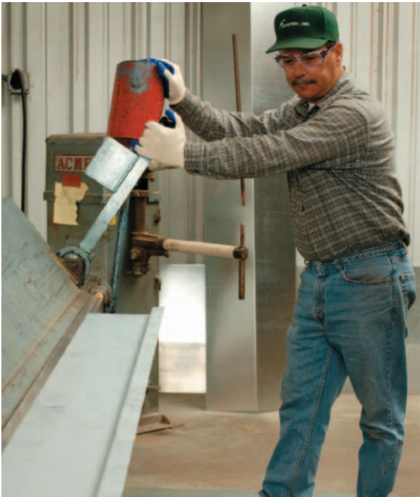
Figure 29-11 Press Brake Taking Form A press brake forms sheet steel.
